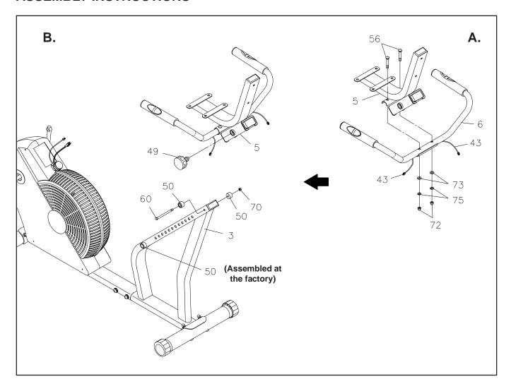
**NOTE:** Be careful not to damage the **PULSE SENSOR WIRES(43)** when attaching the **HANDRAIL(6)** and the **SEAT FRAME(5)**.
